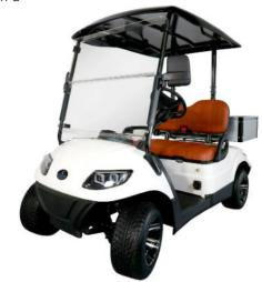
All Cruise® Car vehicles are standard in white with painted black top and stitched brown vinyl seating. Standard safety features include four-wheel hydraulic disc brakes, electronic motor brake, seat belts, headlights, taillights, signals and a folding hard poly windshield.
