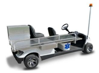
All Cruise® Car vehicles are standard in white with painted black top and stitched brown vinyl seating. Standard safety features include four-wheel hydraulic disc brakes, electronic motor brake, seat belts, headlights, taillights, signals and a folding hard poly windshield.
