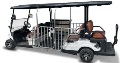
All Cruise® Car vehicles are standard in white with painted black top and stitched brown vinyl seating. Standard safety features include four-wheel hydraulic disc brakes, electronic motor brake, seat belts, headlights, taillights, signals and a folding hard poly windshield.
